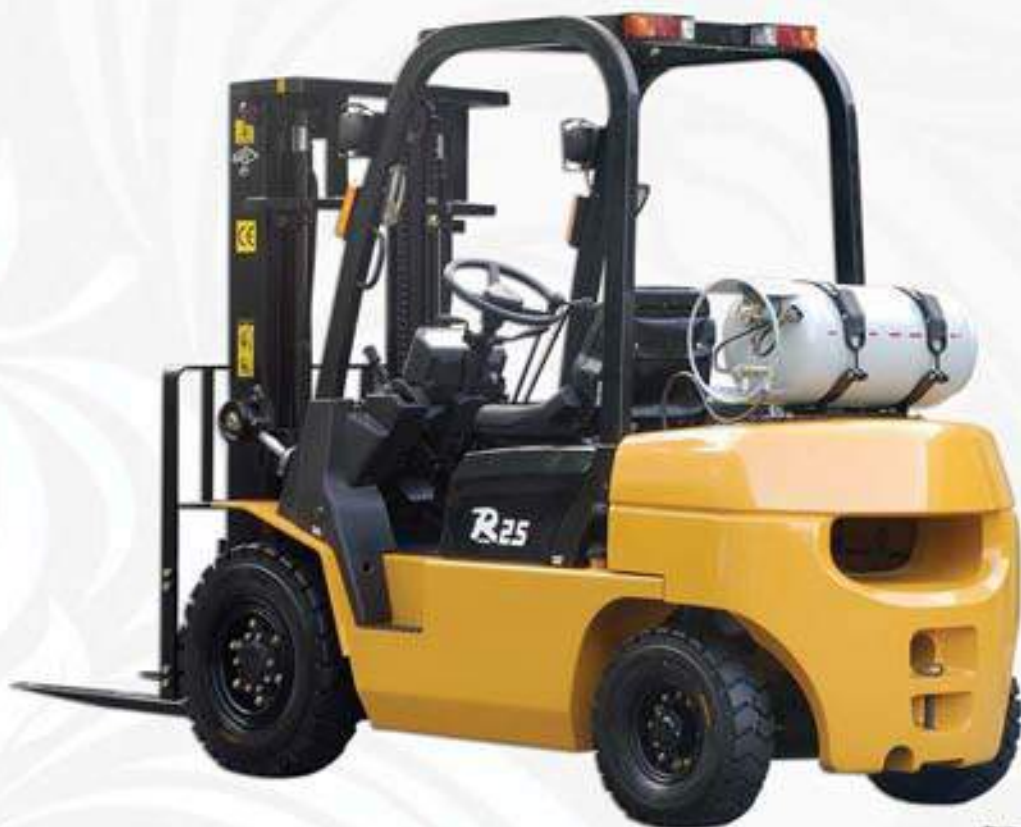
CPQD30N-RW11 Forklift Nissan H25 gasoline 3.5 t, 4.5 m Упқ 42030
